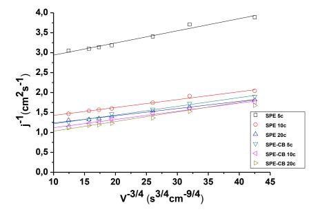
Fig. 2. Dependence of the current density on the flow rate for different electrodes
