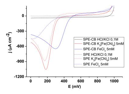
Fig. 1. LSV of LSV of K<sub>3</sub>[Fe(CN<sub>6</sub>] and FeCl<sub>3</sub> on SPE and SPE-CB in HCl/KCl 0,1 M solutions
